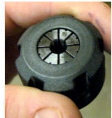
Spindles: snap collet into nut, then flip it over to ensure it is snapped in securely
