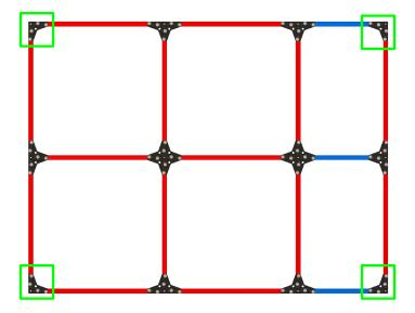
Insert **6x** T Joints around the perimeter of the enclosure top and fasten in place.
