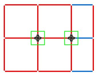
Insert **4x** L Joints on the corners of the Enclosure Top and fasten in place.
