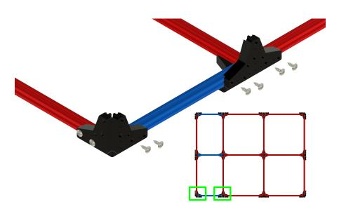
Attach **9x** 30.5" Sticks to the four corners of the enclosure along with the 5 open slots on T Joints around the frame.
