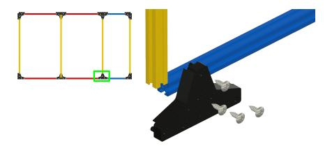
Attach an L Joint to the bottom corner of the enclosure.
