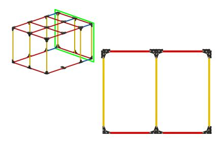
Attach an L Joint to the base of the enclosure.
