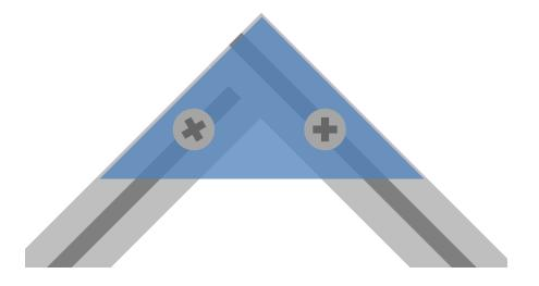
To make assembly even easier-we've manufactured our own ShopBot-cut joinery for V-slot extrusion. They will be referred to by the letter of the alphabet that they most closely resemble.
