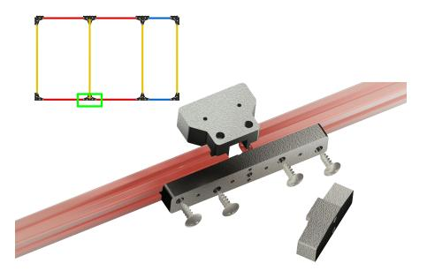
Now attach the connector holder at the bottom front of the enclosure frame to the front piece of extrusion on the base frame using 2x #14 x 3/4" Truss Head Screws.
