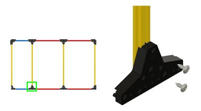
Attach 2x 19.5" Sticks to the base of the enclosure frame.
