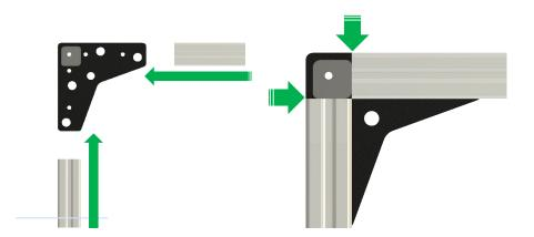
You'll just need to drop the joint into place on the extrusion and tighten the bolt-heads to lock the structure in place.
