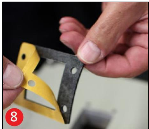
Remove the foil off the one-sided self-adhesive gasket.
