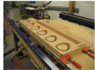
Beacon Custom Woodwork's Shopbot CNC router allows it to machine complex parts, such as this speaker housing.
