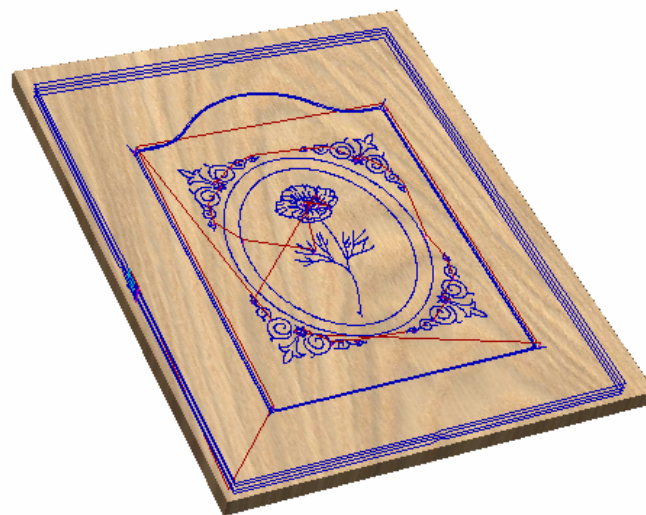
3D Preview showing the calculated toolpaths
