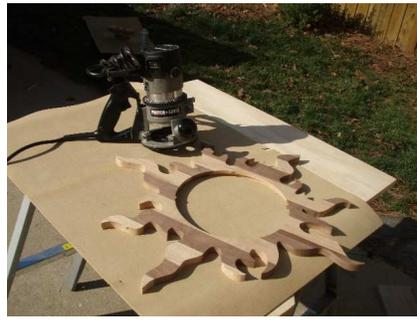
The entire outside of the project is routed with a 1/4" roundover bit. The only edge that is not rounded over is the rabbit on the backside that the mirror drops into.
