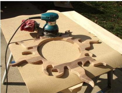
Sand all the edges and faces to ensure the grain is smooth. A random orbital sander works great because one does not have to follow the direction of the grain while sanding.
