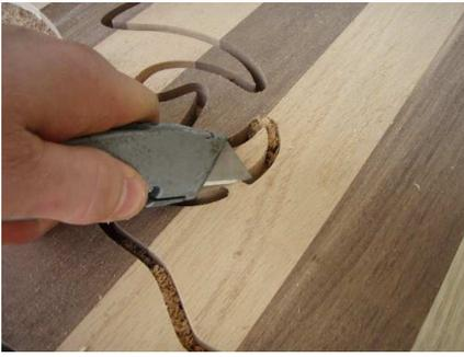
Tabs are use to hold all the pieces to the scrap wood attached to them. Use a utility knife to score these edges. Never try to push a piece out without cutting the tab, it will tear the grain on your project. Sand remaining tab flat.
