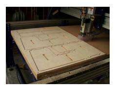
Once the file is complete check to make sure the profile pass went all the way through the work piece and you can see the table surface underneath. Make sure the project is held down in place with your choice of hold down before running the file.
