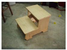
Dry fit the parts to make sure they all fit together. Also take a sander to all the pieces and knock down any sharp edges.
