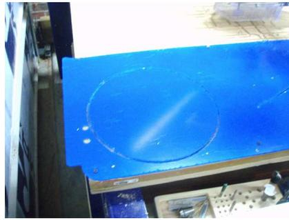
Plastic need to be cut at a much higher RPM. Note the feeds and speeds in the file and also follow manufactures of the plastics recommendations.
