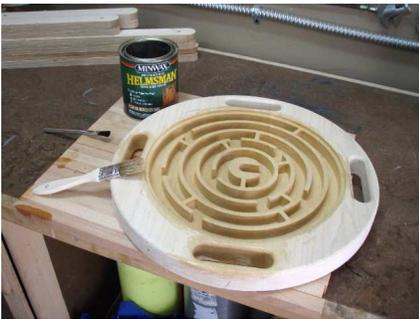
Finish the material with several coats and make sure all of the grooves are stained, once the glass is installed you will not be able to get back into this area.
