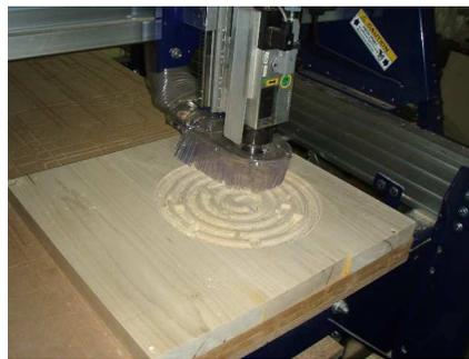
Keep your eye on the project, anytime you are cutting a file for the first time make sure it is dialed in for the machine you are cutting it on.
