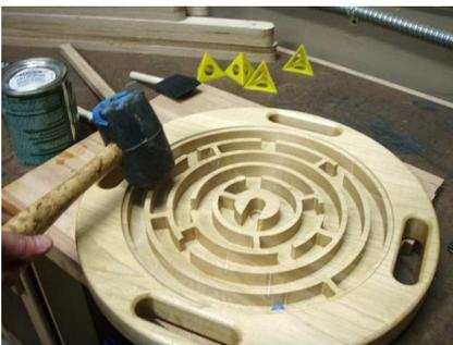
A rubber mallet may be needed to push the glass or plastic down into the groove. Try not to scuff the material.
