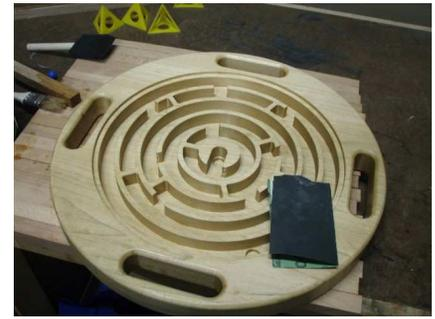
Before applying the finish it is a good idea to route all of the handles and outside edges of this project with a round over bit. This will make the project more comfortable to handle.
