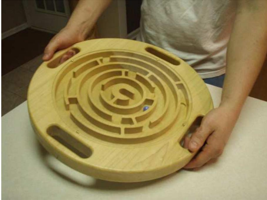
As seen above the marble game is complete. There are four screws, once centered over every handle. Some small brass screws were used to help add to the “eye” appeal of the project. Remember to route or sand all the handles so it makes the project more comfortable to use. One idea is to cut two of these projects and have races to see who can complete the puzzle before their competitor.
