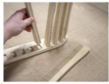
Place the pieces into the pockets on the chair sides. Notice the joints are hidden due to the routed edges.
