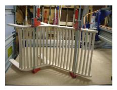
It can be usefull to get a 3rd hand from a innocent bystander to help line up all of the slats into the pockets. Once this has been done clamp the project together and let the glue set up overnight.
