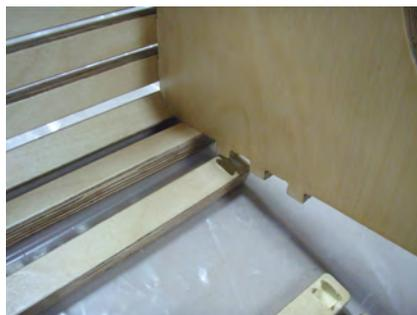
If parts are snug going together, tap with a rubber mallet into place. Make sure a good amount of glue is in the pocket.
