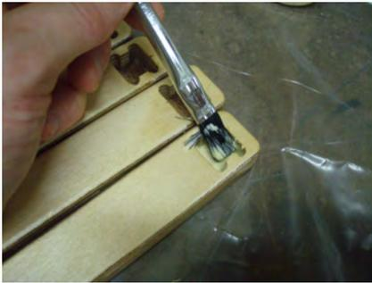
Use a good amount of glue in each pocket. Take a small brush or your finger and cover all of the surfaces in this joint. It is better to have a little extra glue that squeezes out then not enough and the basket falls apart. Squeezed out glue can be easily wiped off.
