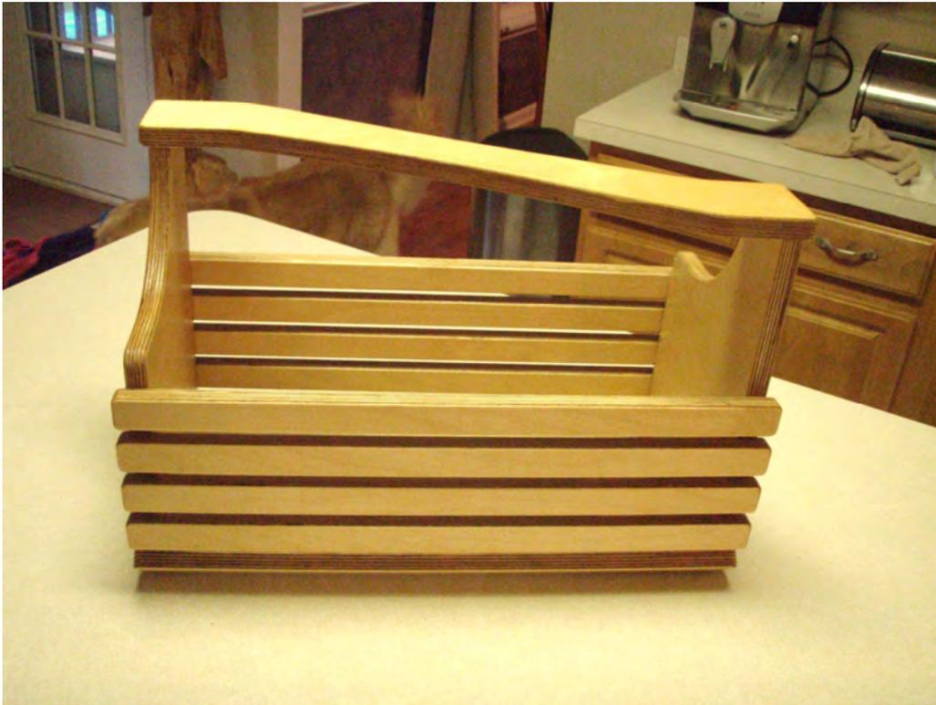
The project will take shape and square itself as you assemble the slats. Wipe off any glue runs or glue that squeezed out of the joints. Double check the project for any spots that might have been missed during the finishing project. If you desire, add another coat of polyurethane to the outside of the basket to really make it shine. This basket can serve for many different jobs around the home and makes wonderful Christmas gifts.
