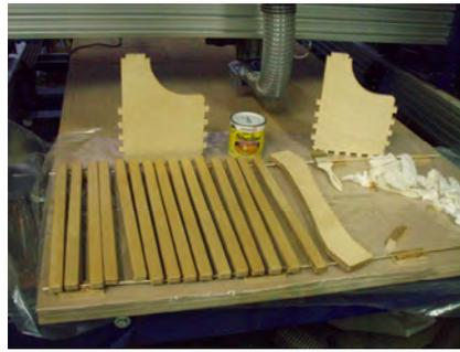
Make sure you have fifteen slats, two end pieces and a handle. Get at least two coats of a polyurethane of your choice on each part before assembly. Try to keep the polyurethane out of the pockets and off the tenons on the end pieces.
