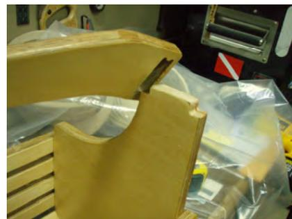
The last step is to glue on the handle. Fill the pockets with glue, tap into place, flip basket upside down and let it sit for 30 minutes.
