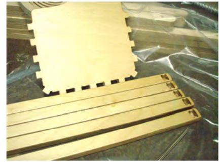
To start assembly you will need five slats and the two end pieces. Pay attention to the pictures to see the orientation of the end pieces. Failure to follow this layout will result in your handle not fitting.
