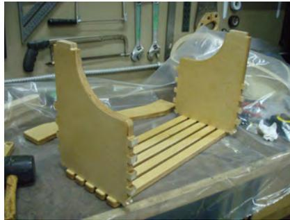
Fill all the tenons on the five bottom slats. Then install the bottom pieces into these slats. Use a rubber mallet to help push it all together. \*\*Note the direction of the end pieces and the handle in the background, if you have the end pieces backwards at this point, the handle will not fit.\*\*
