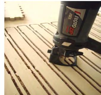
Removing tabs with a utility knife works great. However if you have access to a RotoZip tabs can be removed a lot faster. Never try to push a piece out without cutting the tab, it will tear the grain on your project.
