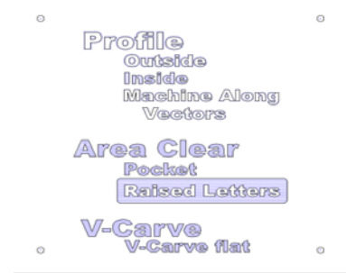
2D view of the toolpaths with the Solid box checked. Does the bit go deep enough into the corners?
