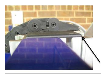
Install end cap with a firm, even pressure until flush with surface as shown.
