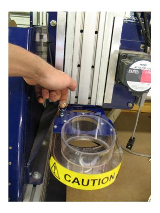
To attach the dust foot, you will need to pull the pin on the foot as shown and slide it onto the dust foot bracket. For normal installations with a spindle/router already installed, you will need to lower the bracket below bthe spindle/router to provide interference-free installation of the dust foot.
