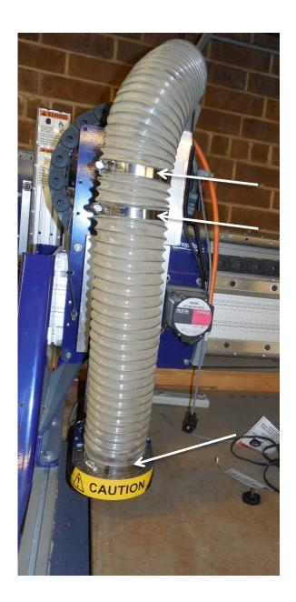
Using the three hose clamps provided, connect your 4"dust collector hose to the dust foot and to the dust hose bracket as shown. Leave enough slack in the hose above the dust hose bracket to allow full travel of the machine. Check full travels to ensure the hose does not bind or get caught anywhere. A good option for setup has the hose fastened over the center of the table to allow for the most travel with the least amount of slack.
