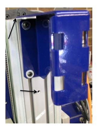
Slide the bracket onto the rail. Once the bracket is positioned at the top of the Z rail, tighten the screws into the T-nuts securing the dust hose bracket into place. Be sure not to install the bracket on top of the knob hole.
