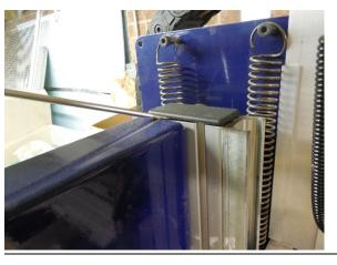
This is done by gently prying up the cap with a screwdriver. Keep the cap level as you pry it up by using the screwdriver around all of the edges. The cap should come off straight up. This will prevent the legs of the cap from being stressed and potentially breaking its prongs.
