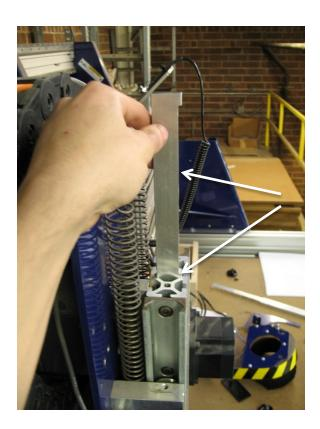
Orient the front dust bracket rod so that the large notch in the rod is to the front and top.
