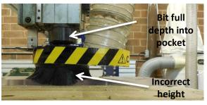
Setting the dust foot to the correct height is dependent on the material thickness and length of bit. Set the height of the dust foot equal to the material thickness, minus 1/8" above the tip of the bit. This allows the bit to reach full depth of cut and only deflects the dust footing slightly. If you know the max depth that will be cut on the part (when you are not cutting all the way through), you can set the height lower accordingly to maximize suction.
