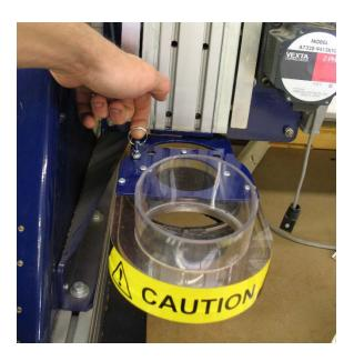
When changing bits, loosening the knob allows for the dust foot to drop out of the way. If there is not enough height, or the dust foot is otherwise in the way, you can remove the dust foot using the quick release pin. Pulling up on the quick release pin and sliding the foot out allows for quick and easy removal.
