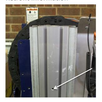
If you are retrofitting to an older machine, a hole for the knob will have to be added into the Z rail using a 5/16-18 drill and tap set. Use the drawing at the end of this document to measure the proper hole location. Make sure it is oriented according to the document in order to line up with the shaft slot running down the center of the rail.
