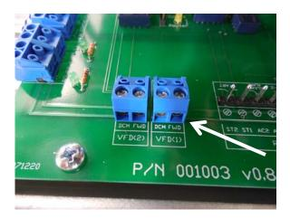
Remove the two pin terminal block from the control board marked "VFD(1)" and replace it with the two pin terminal block on the wiring harness.
