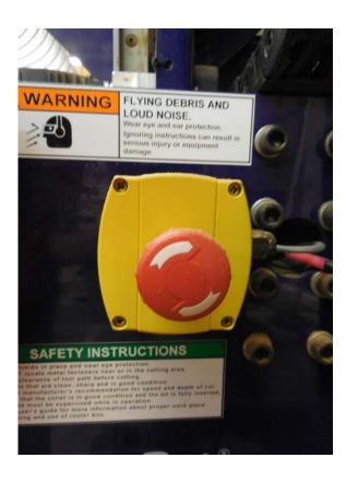
The separate emergency stop switch also comes fitted with a terminal block that plugs into the control board. Power for the router or spindle is routed through the PRSalpha control box safety controls so that activating the E-stop by hitting the red button will stop the movement of the carriages and stop the router or spindle. We suggest mounting this to the gantry on your machine in an easy-to-access location.
