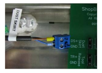
Bring the cable marked "dust skirt" into the control box. Route the dust skirt cable to the ATC interface board. Then connect the blue three pin terminal block to the location marked "dust skirt."
