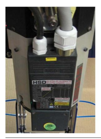
Plug the cables into the mating plug of the HSD spindle and secure the socket head screw so that the plugs are locked in place. Route the cabling from the spindle through the Y axis E-chain into the control box and over to the left side of the ATC interface board. The spindle cable should already have the terminal blocks ready for installation from ShopBot.
