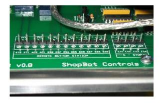
This is the PRSalpha control board before the terminal block from the three button pendant is attached. Note that the terminal block for the separate E-stop is also not attached yet.
