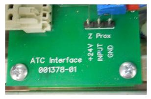
Inside the control box, route the proximity cable to the lower edge of the ATC interface board. Connect the blue three pin terminal block to the location marked "Z Prox."
