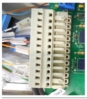
Find the female Wago on the board where it is printed as "Spindle Sensor Cable." Then, connect the male Wago connector into the ATC interface board.
