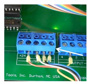
Tip: Terminal blocks are placed on straight pins soldered to the board. In order to remove them, simply apply force straight up to lift them off of the pins.
