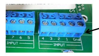
Remove the five pin terminal block from the portion of the control board marked with the following inputs: 4, 3, 2, 1, and Gnd. Replace it with the right most five pin terminal block on the wiring harness.
