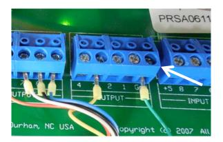
Remove the five pin terminal block from the portion of the control board marked with the following outputs: 4, 3, 2, 1, and Gnd. Replace it with the middle five pin terminal block on the wiring harness.
