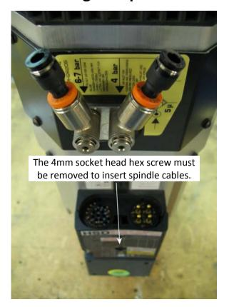
Locate the spindle cables. Remove the small socket head screw from the front face of the spindle's plug (4mm hex wrench needed).
