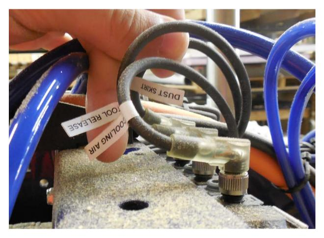
Locate the row of solenoids mounted on the upper Y axis E-chain bracket. Connect them with the appropriately marked cables provided. After you connect the solenoid with its matching cable, route these cables through the Y axis E-chain and into the control box.
