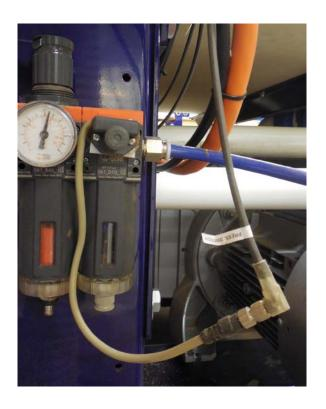
The pressure switch is located on the primary air regulator where your compressed air input attaches to the tool. You will use the threaded pressure switch cable to attach to wire coming out of the pressure switch. Route the other end with the two pin terminal block into the control box.
