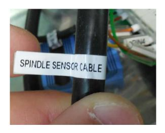
The other long connector should be labelled as the spindle sensor cable. This is a male Wago connector and will connect into the corresponding female piece on the ATC board.
