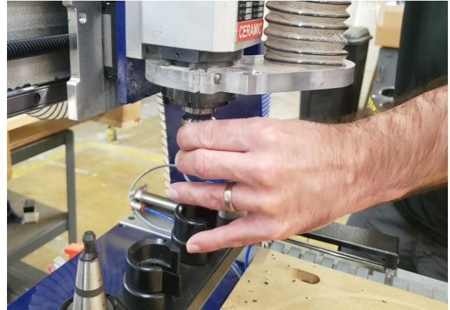
Insert a tool holder into the spindle
