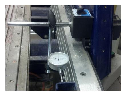
Picture of a Y axis setup with the indicator base attached to a side plate and the indicator against the Y motor. Push/Pull on the YZ car in the Y direction.
