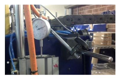
The following two setups have the base attached to a table leg and the indicator is touching an upside down 1/2" bit to measure deflection at the bit in the X and Y directions. Push/Pull on the bit or collet nut directly at and away from the indicator.
