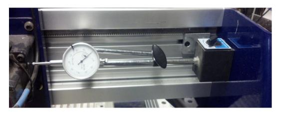
This setup is used to measure play in the Z axis in the vertical direction. The base is attached to the YZ car and the indicator touches the top of the Z extrusion. Grab the spindle or Z extrusion and Push/Pull in the Z (vertical) direction.
