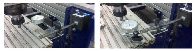
The first 3 setups are directly aimed at the pinion/rack adjustment. The last two, which will show lateral deflection at the bit, can show play in the lower YZ car bearings, play in the Z bearings or a loose spindle connections. To gain an accurate assessment at the bit, all play must be removed in the first three tests prior to setting up for the last two.
