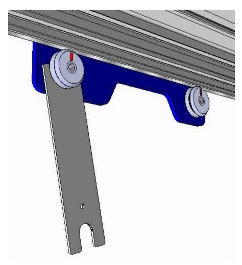
Start with the Red mark at 12 o'clock Rotate the shaft in a clockwise direction in small increments until it fully engages the rail. Try to rock the YZ-Car back and forth from the front to make sure the wheel is tightly engaged and there is no wiggle, but do not over-tighten.
