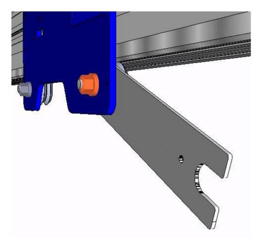
When you have each wheel adjusted, hold the flat wrench while locking the wheel in position, tighten the nut securely.
