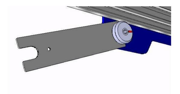
Check your adjustment over the entire rail. You should not be able to stop the wheel from turning with finger pressure. It can be tight enough to produce a slight amount of resistance to rolling. **Do not over tighten**.
