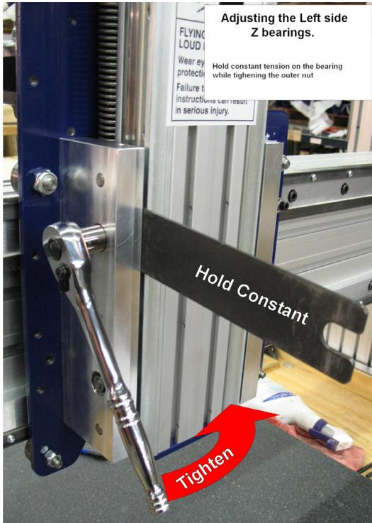
After adjusting the eccentric bearing to the proper tension as instructed above, hold the position of the bearing constant with the flat bar wrench while using a 13mm socket wrench to tighten the outer nut.
