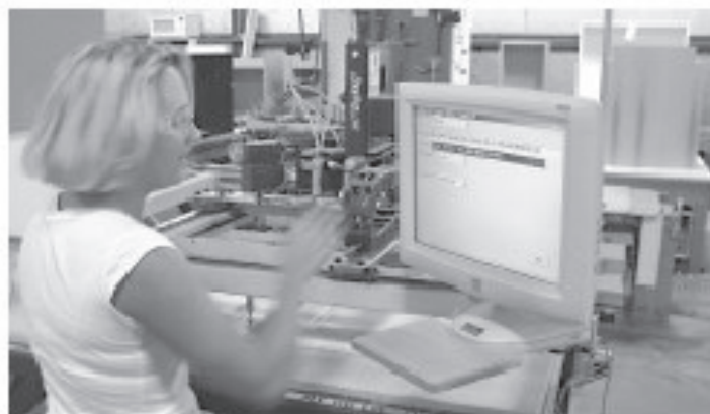
Programming for boring on the ShopBots is done on the screen. This was more efficient than using the keyboards.
