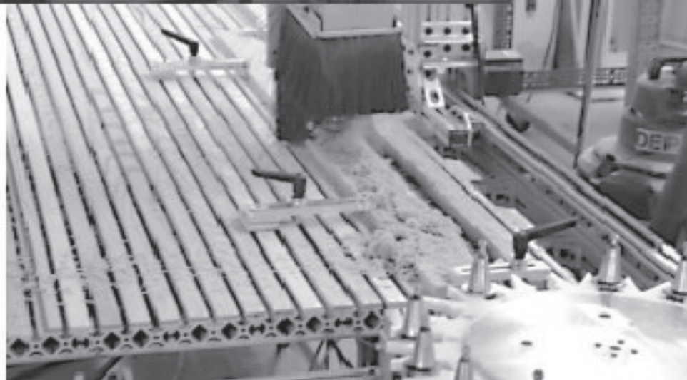
One of two Shop Bots used for making components. This one is making a long, thin part. Machines can be used for small quantities or special orders.
