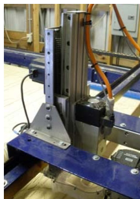
PRS Retro Z Axis with 2.2hp spindle on PRT with single-piece Y car
