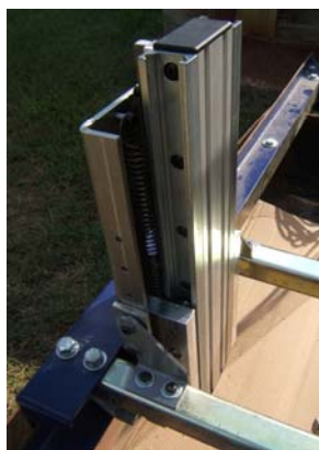
PRS Retro Z Axis on PRT with strut-style Y car
