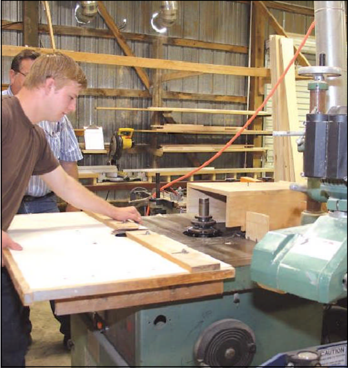
Dual purpose — When the shaper table is removed and an air-powered jig added, arched doors can be cut with limited equipment.
