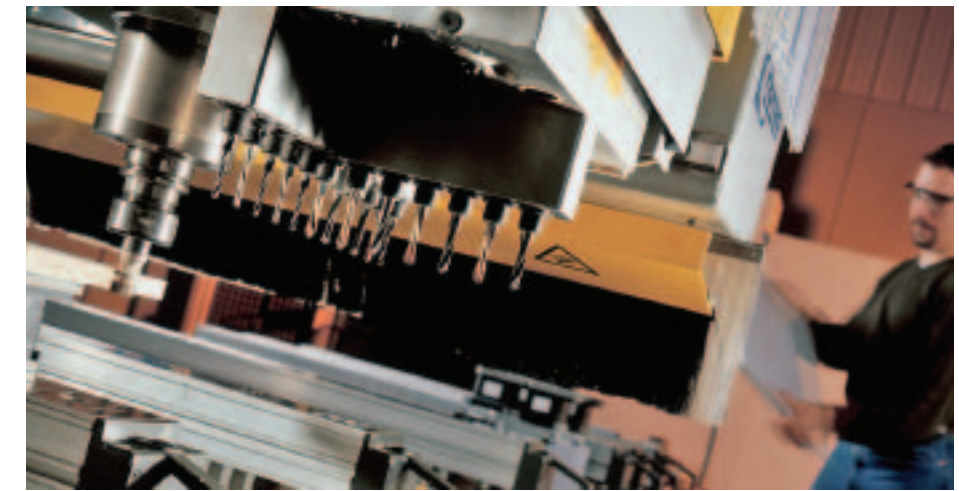
A Homag Group employee operates a Homag BAZ series stationary processing center that routs, grooves, bores, and applies and finishes edgework.
