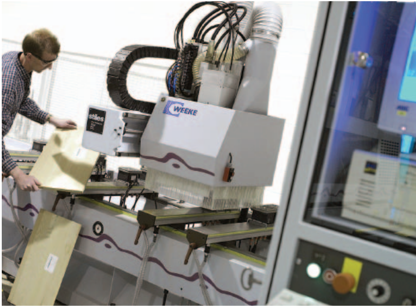
The Weeke BHP 200 nested-based CNC machining center is built for both small and large manufacturing operations. It's designed for routing, boring, and grooving of flat components that have been nested into full sheets of material.
