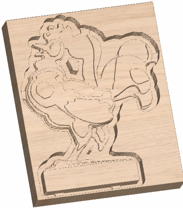
Preview of the Z Level Roughing Toolpath
