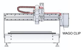
All ShopBot models have a wago connector for attaching several Z Axis Zeroing Devices.
