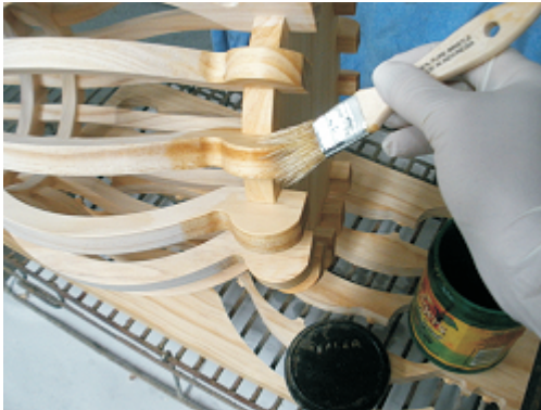
Applying thinned SealCoat
