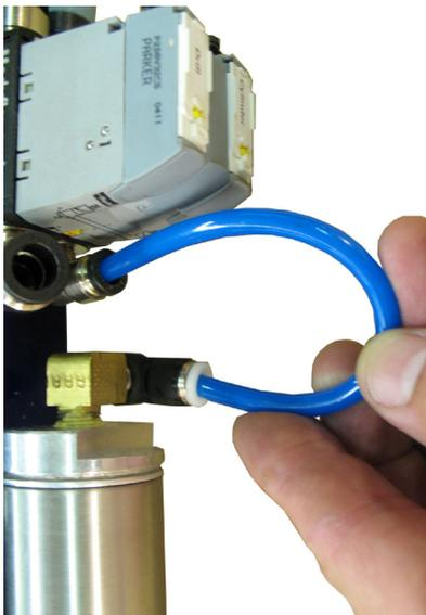
Use 1/4" tubing to connect the 1/4" push-in connectors.
