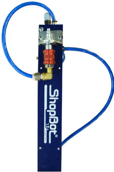
Connect the upper push-in of the dual valve to the 1/2" push-in of the air supply assembly using the length of 1/2" tubing that was originally removed from the SV air drill.
