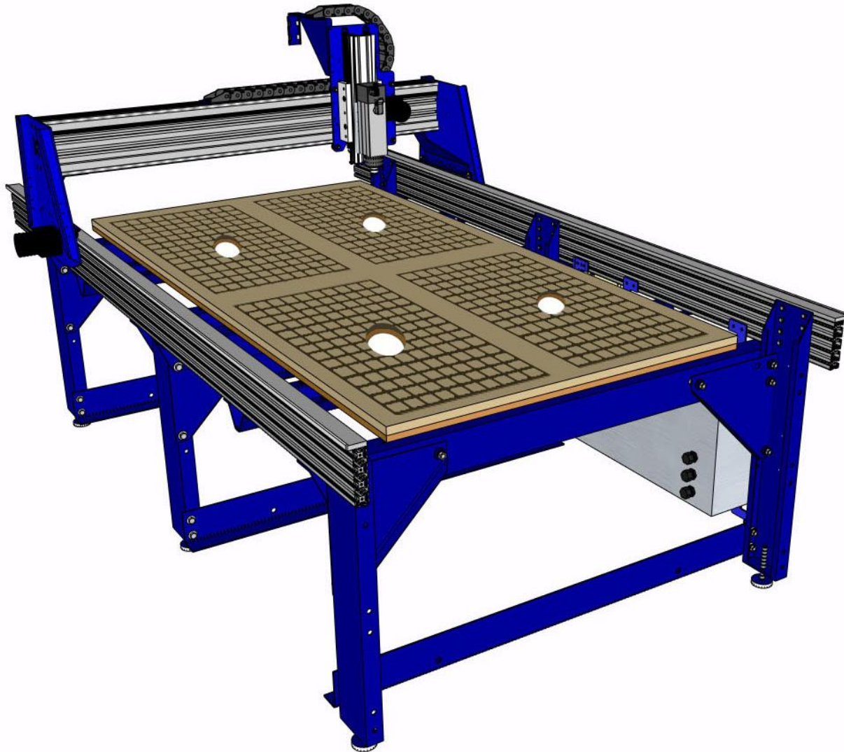
Standard Plenum Hole Placement
